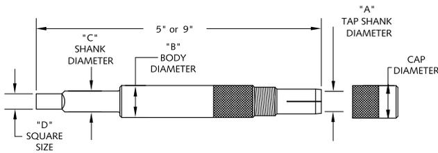
The tap shank enters the hole and is locked into a square in the bottom of the hole. The tap is then secured by hand tightening the compression cap.
