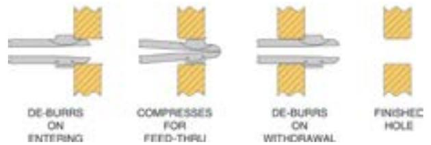
**System II** - which has a "bullet nose," is used for applications in which only the **back side** of the hole requires de-burring.
