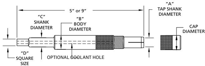
The tap shank enters the hole and is locked into a square in the bottom of the hole. The tap is then secured by hand tightening the compression cap.
